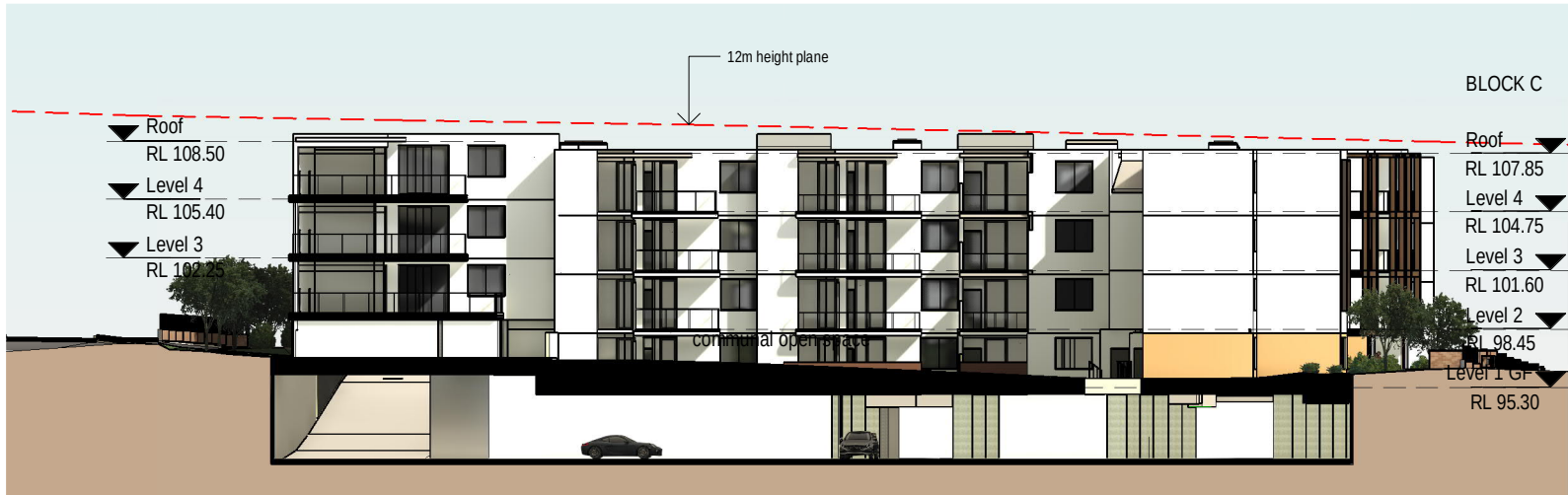
1 Sectional Elevation 3 - Block C 1 : 400
