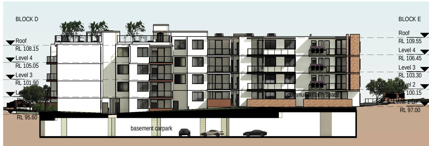
2 Sectional Elevation 4 - Block D & E 1 : 400
