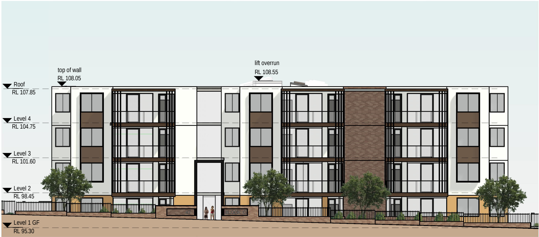
1 NORTHEAST ELEVATION BLOCK C ENTRY 1 : 200
