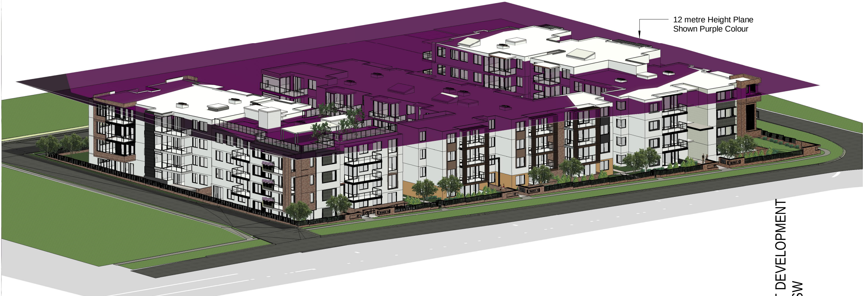
1 12m HEIGHT PLANE view along Ingleburn Rd looking West
