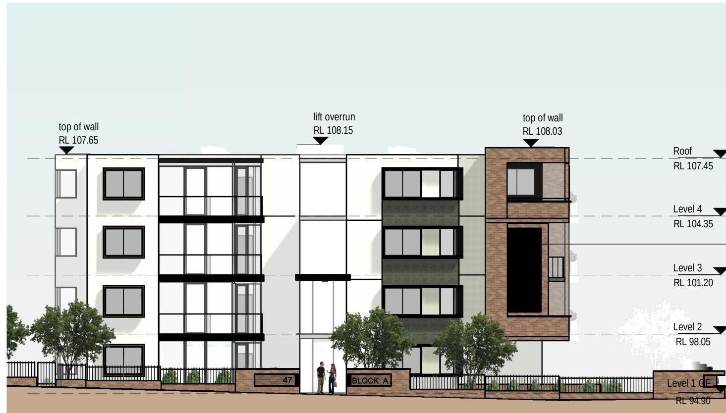
1 NORTHEAST ELEVATION BLOCK A ENTRY 1 : 200
