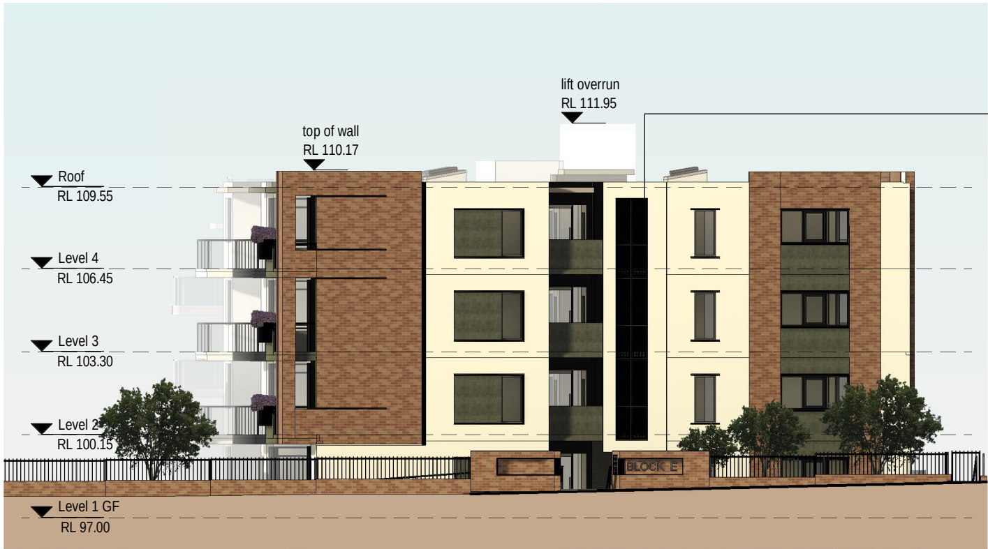
1 SOUTHWEST ELEVATION BLOCK E ENTRY 1 : 200
