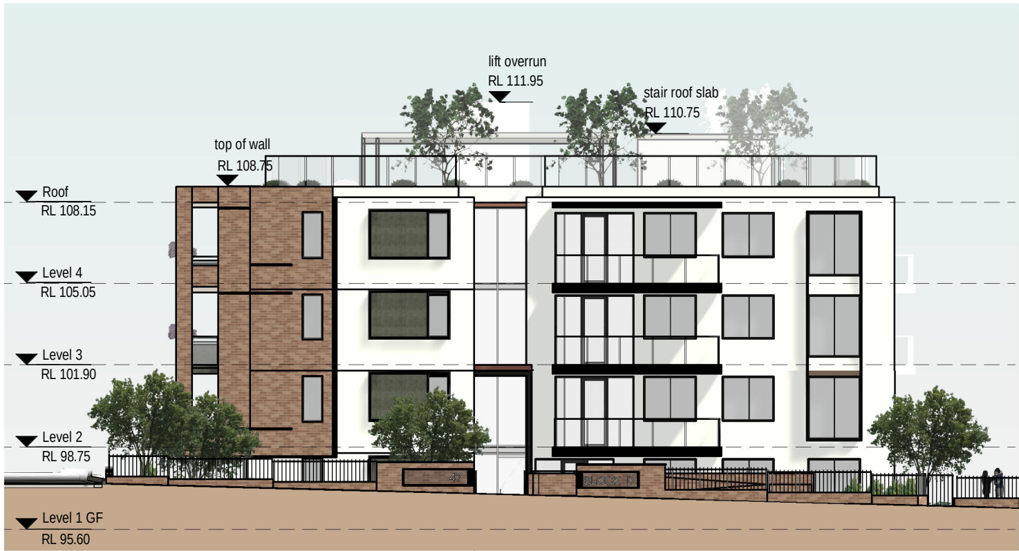
2 NORTHEAST ELEVATION BLOCK D ENTRY 1 : 200
